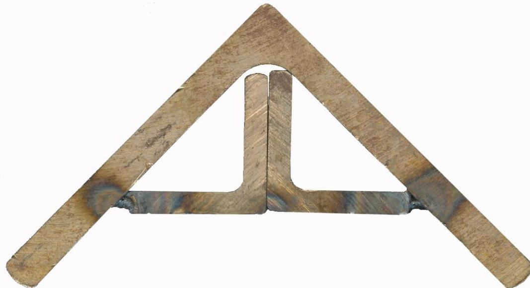
**Cross-section of 4-inch angle-iron bar with 1 1/2-inch stiffeners welded inside (to scale).**
