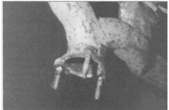
**5.28** The new stud is now welded in place, with strength said to be up to 85% as good as original. This feature is a real time-saver for busy muffler businesses.
