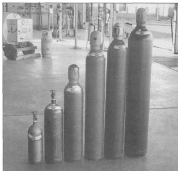
6.16 Argon bottles are available in a number of sizes, depending on whether you are trying to make your TIG setup portable or not, and how much welding time you need. Shown here, from left, the sizes are: 20, 55, 80, 125, 154 and 248 cubic foot.
