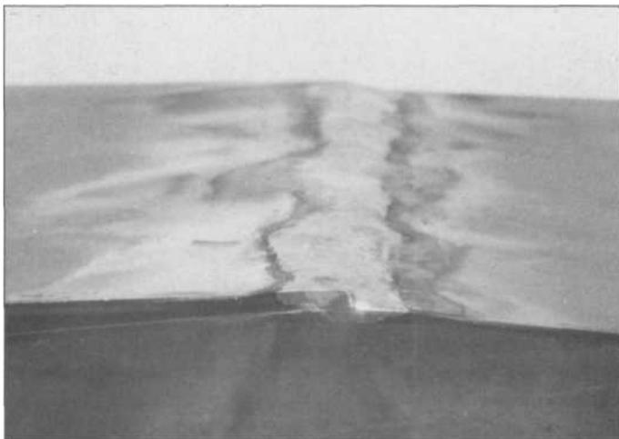
**3.36** End view of a brazed lap joint, showing how the brass flows in between the plates with capillary action, much as solder does when applied to a hot copper pipe. The base metal must be heated to the point where *it* melts the rod, not the torch.
