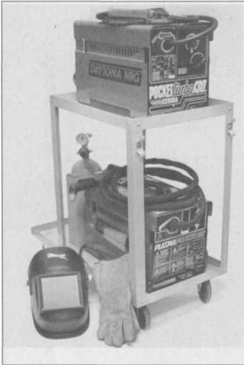
**2.28** Where the really complete home/shop setup was once an AC arc welder and a set of gas torches, today more shops utilize a MIG welder and plasma cutter. This welding cart features a gas-shielded 130-amp MIG and a plasma cutter capable of cutting up to 3/16-inch material, and both machines operate on household 110V current.
