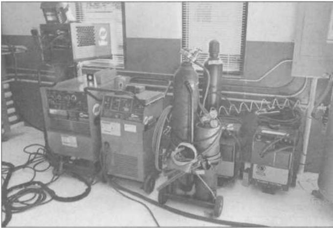
**2.3** The welding corner of this well-equipped race-car prep shop holds a variety of equipment, from a large TIG machine at left (with cooling unit on top), to a heavy-duty plasma cutter, oxy-acetylene cutting/heating/welding outfit, and two small plasma cutters. Not shown here are the two MIG welders in use elsewhere in the shop.
