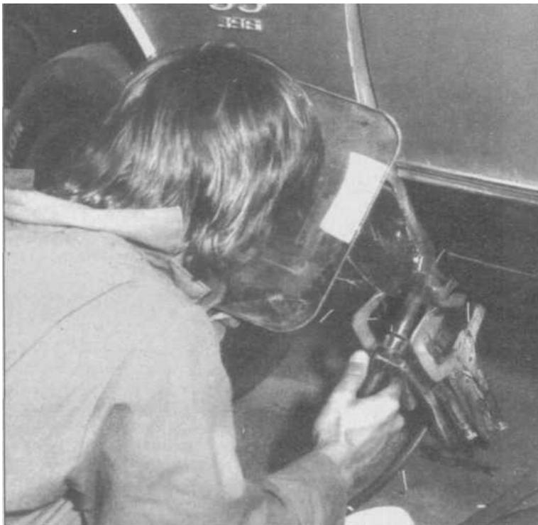
**5.55** Don' be tempted by the low spatter of MIG welding to just shut your eyes when tacking body panels. If you need speed and convenience while tacking, use a hand-held safety-shield with lens as shown here. Weldor here has long sleeves, but should have gloves on and a turned-around hat to protect his hair from hot spatter.
