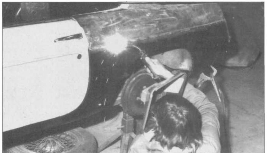
**5.1** The use of wire-feed MIG welding has expanded greatly in the last ten years to encompass body shops, muffler shops, race-car builders and home hobbyists as well as the industrial production work it was designed for. It has advantages of speed, simplicity, cleanliness, and the ability to work well on thick and thin materials.
