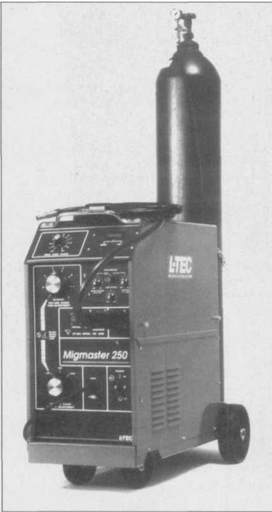
**5.3 For the larger-scale shop, the heavy-duty 220V machines like this Migmaster 250 offer more amperage, more amp settings, higher duty cycles, and various extra features for timing various weld functions.**
