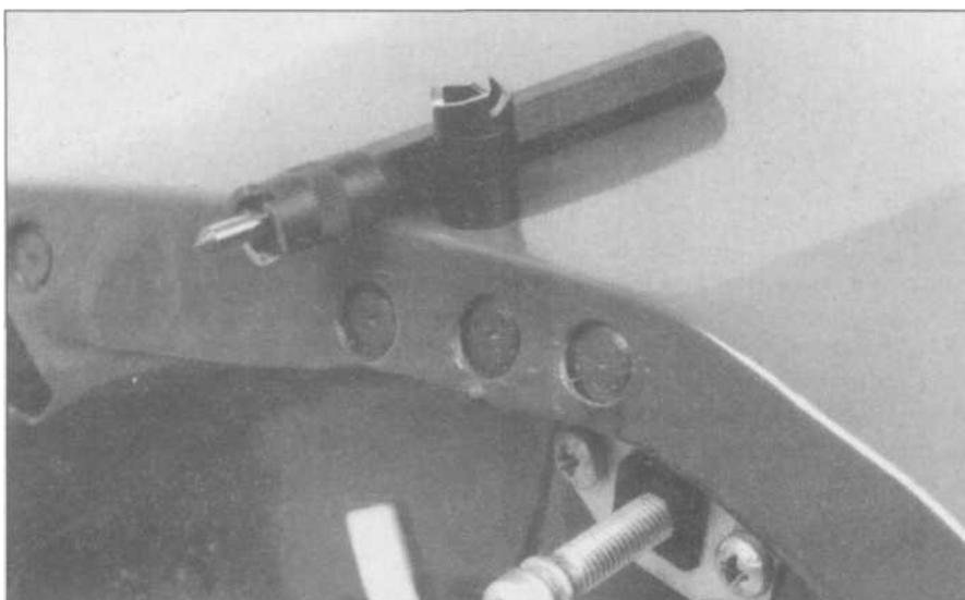
8.20 For Eastwood offers a similar tool for removing spot welds which features a hex-sided drive end, so it can't slip in your drill chuck.
