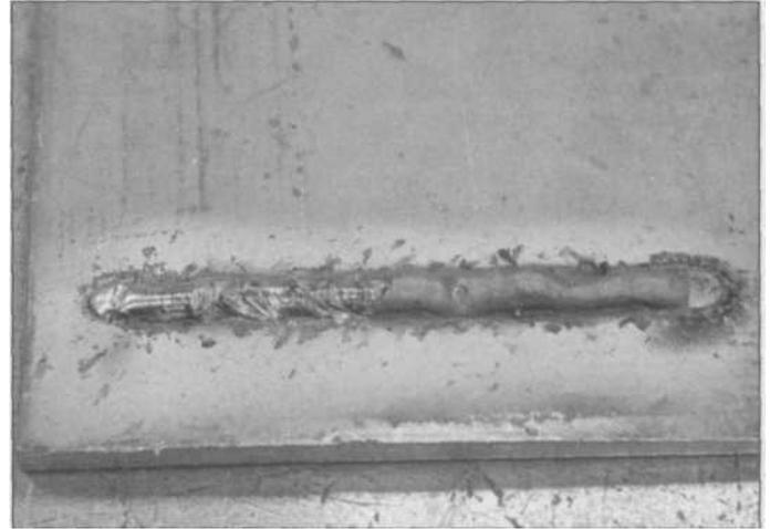
**4.14** At right on this bead, you can see the dark gray slag coating covering the weld. The portion at the left has been chipped off to reveal a bright, shiny weld.
