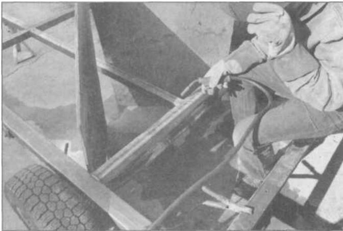
**5.32 Gas-shielded MIGs are not made for outdoor work, but as long as you can keep the wind currents away, they work fine. On this driveway utility-trailer project, pieces of plywood are used as wind shields while welding.**
