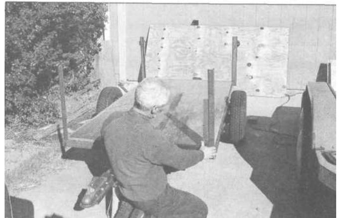
9.27 Four posts of heavy 1x2-inch angle-iron were welded on, one in each corner, as supports for the plywood sides. After welding, all were checked with a square.
