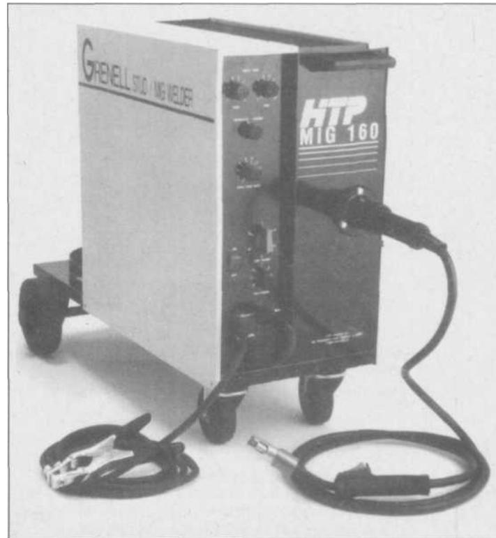
5.22 Above the 140-ampere range, you are into the 220V category of **MIG** welders, with more features and higher duty capacities. This is HTP's **MIG 160**, which can weld up to 5/16-inch steel, has eight heat settings, and is suitable for street rod shops, muffler shops, or farm use.
