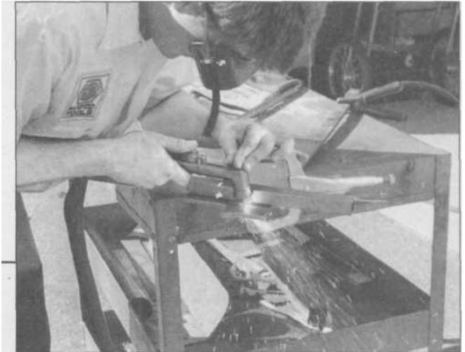
7.1 Plasma cutting can be done outdoors, being very little bothered by wind, makes very clean cuts on ferrous and non-ferrous materials, and produces no smoke and very little sparks. It has become the modern way to cut metal. The operator here should be wearing gloves and a long-sleeved shirt.
