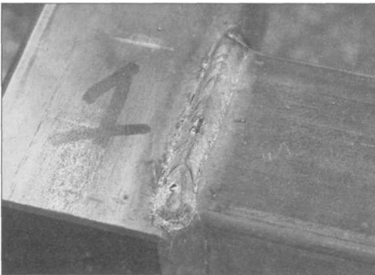
5.45 This production weld by a professional shows how clean and perfect MIG welds should look. The heat-affected area on either side is small, the weld has good penetration, and there is minimal spatter. Heat was evenly played on both pieces of tubing.
