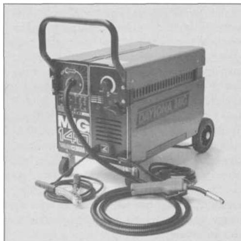
**2.16** Small, portable wire-feed, or MIG, welders have become one of the most popular welding machines for home/shop use. Easy to set up and simple to operate, they produce very clean welds, and models from 100-amp to 140-amp can be operated on household 110V current.
