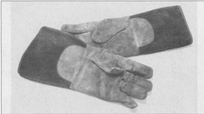
**8.8** A good pair of leather welding gloves will last you for many years, but if you are using oxy-acetylene equipment, keep an extra-clean pair for use with this equipment. A spurt of oxygen on a dirty glove could cause combustion, so don't use these good gloves for handling hot or dirty parts.
