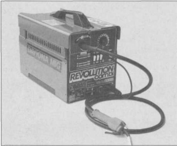
**2.17** Most MIG machines operate with a bottle of shielding gas, but some are equipped to run with flux-cored wire which makes its own shielding gas as it arcs, making the process more suitable for outdoor and drafty situations. This home/shop-sized unit shown is a combination machine that can operate with gas shielding/solid wire, or the flux-core wire.
