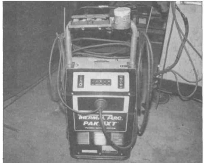
7.18 Hot rodders never leave anything alone. Rugged Thermal Dynamics 50-amp plasma cutter used in a rod shop has been modified with the addition of a tubing rack and box on top to hold nozzle dip and plasma consumables.
