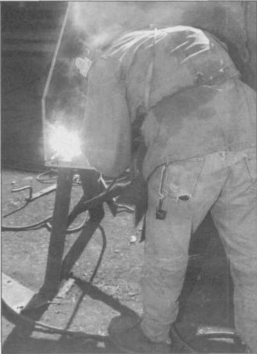
**4.15 The arc spatter and radiation are dangerous. Do not allow any bystanders to observe the arc while you are welding. Also, notice how much smoke is around the weldor's helmet here. The fumes are dangerous and you should have an electric fan of some kind to blow it away from you when you are welding in a corner like this.**
