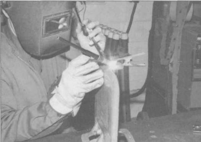
**2.24** While TIG or heli-arc welding is considered by many to be the most *controllable* welding technique, it takes more practice than any other. You have to learn to manipulate the torch with one hand, the rod with the other, and the amperage control with your foot on a pedal. There are no sparks, spatter or slag. Here an aluminum frypan's handle mount is being repaired. The heli-arc welding didn't even bother the non-stick coating on the other side!
