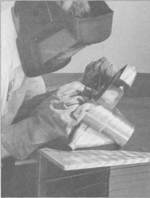
**6.39 TIG welding is especially helpful in situations like this race-car suspension upright, where you have thin chrome-moly plate and tubing, and need total heat control. If you burn through on a job like this, the whole part may have to be scrapped.**
