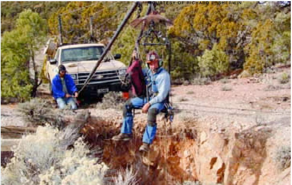
Scott Altenbach prepares for a descent into a mine shaft. Note the rock guard located above his head that has deflected rocks that have been inadvertently knocked loose during internal surveys.
