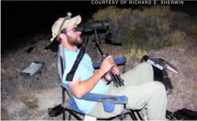
Quality night-vision scopes can be powerful tools at some mines where the size of the opening limits the functionality of other methods.
