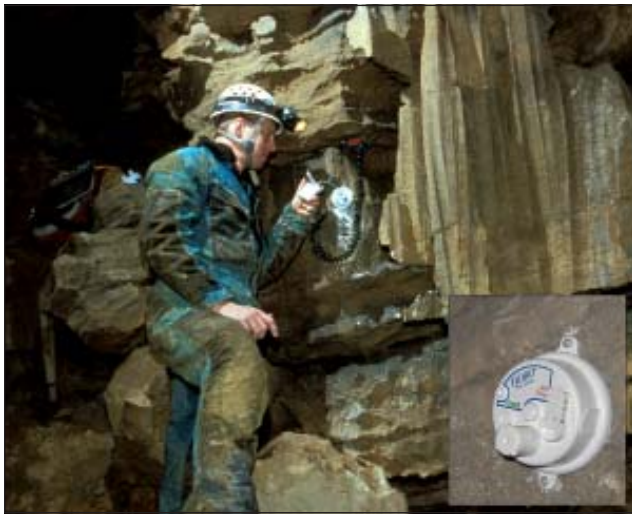
Figure 2. The author getting calibration temperatures at a datalogger in Saltpetre Cave. Inset is one of the Onset Computer Corporation HOBO Pro™ temperature/humidity dataloggers used in this study. Photos by Elaine Acker and Jim Kennedy (inset), © 2000 BCI.
